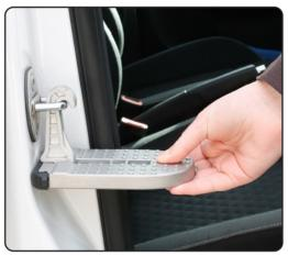
2). Make sure the rubber strip is against the body of the vehicle.
